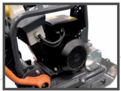
2.2KW ELECTRIC MOTOR & 16KN VIBRATOR
